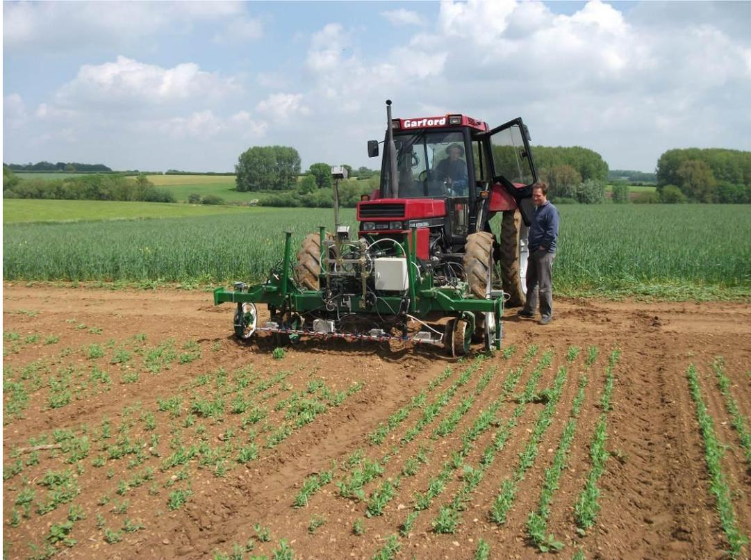
**Fig 9:** Vision guided spot sprayer preparing to travel down one of the 2 m beds.
